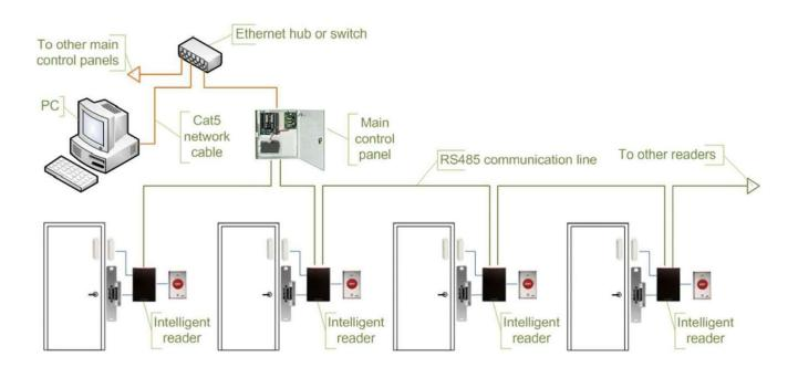
Fully networked and standalone online access control systems. Designed to incorporate all the necessary peripheral devices to control, monitor and have visual display of the plant or building. Complete recording of event information. This system provides the total integrated access control and alarm monitoring system for leading organizations.
